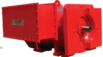
The Joliet Horizontal AC Drilling Motor delivers a continuous 2000HP rating for mud pump and rotary table applications and boasts an impressive intermittent rating of 3045HP for drawworks duty. The continuous rating is at 600 VAC, 1750 Amperes, 45.6 Hertz, 900/3000 RPM, Torque @ Rated Speed: 11,710 (Ft. lb.)
